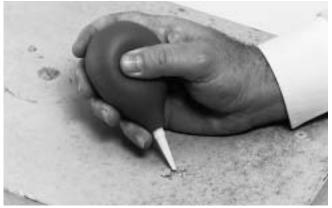
**Cleaning** Air blower cleaning out pin hole before measuring.
