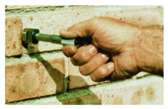
**Measuring** Needle micrometer measuring depth of pin penetration in mortar joint.
