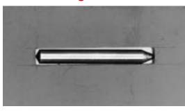
Used steel pin passing through the Go/No-Go gage.
