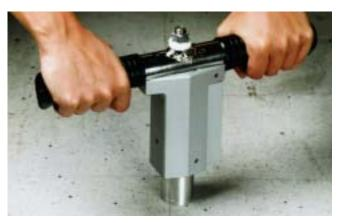
**Firing** Windsor Pin with chuck on smooth surface.
