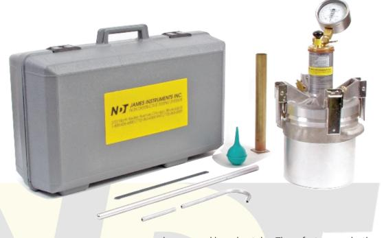
read gauge, and bourdon tube. These features make the James Instruments® ASTM "Type B" Pressure Air Meter the most durable, accurate, rapid and easy to use meter on the market. The pressure gauge is color coded for entrained and entrapped air. The system meets ASTM C-231 & AASHTO T152 standards.
