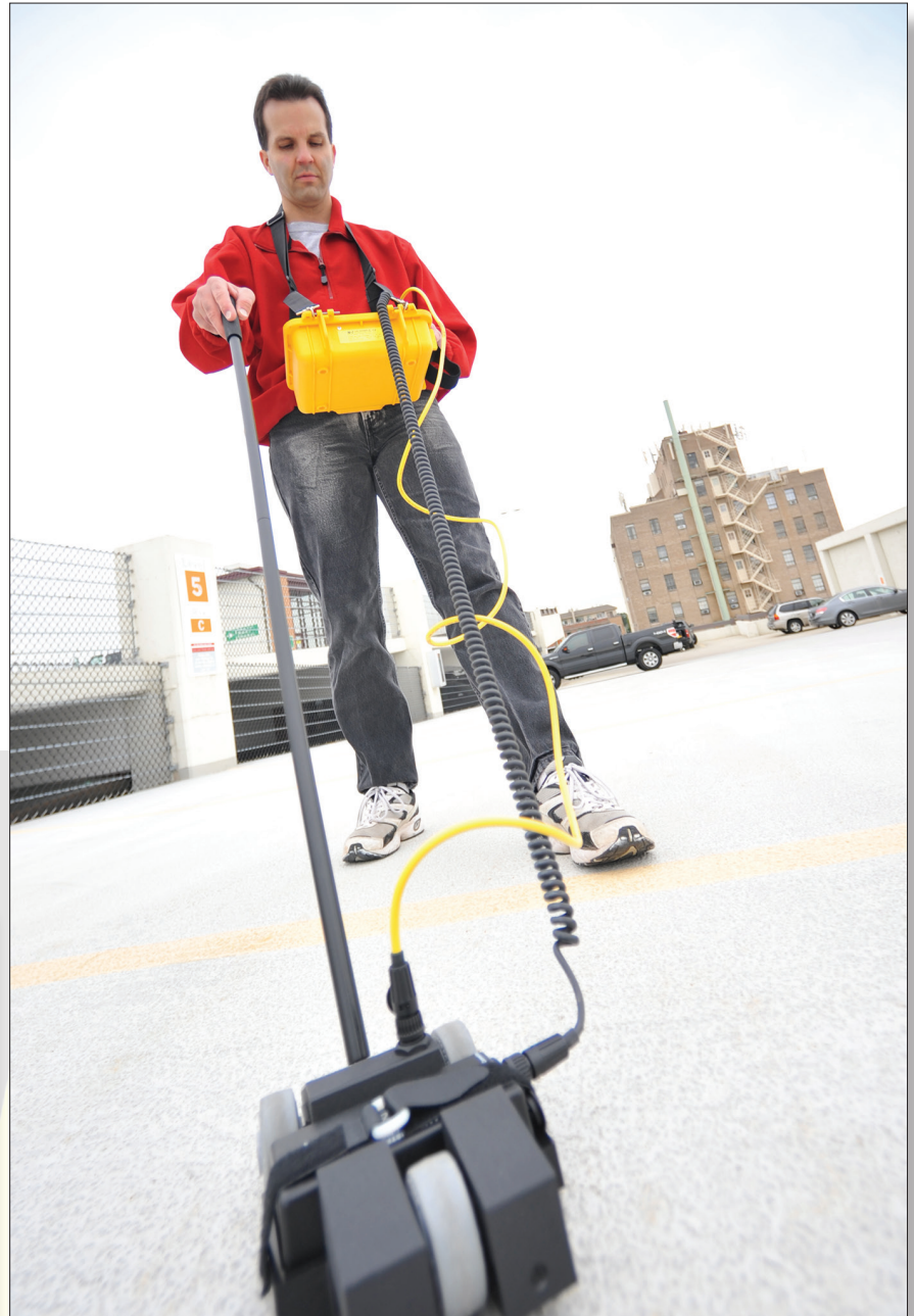
Above, the Rebarscope® is shown with the Rolling Scan cart, used for surveying a large area such as a parking garage. At left, Rebarscope® in a typical application.
