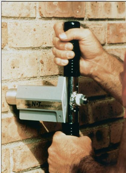
Testing mortar joint on a brick wall (left) with the chuck removed (right)
